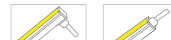
End cap (outlet from bottom direction) End cap (outlet from end direction)
