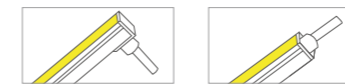
End cap (outlet from bottom direction) End cap (outlet from end direction)
